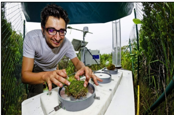
In situ lysimeters to record and follow cloud water interception and retention by liverworts
